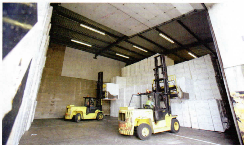
Pulp is moved by clamp truck to a purpose-built warehouse a few meters away
